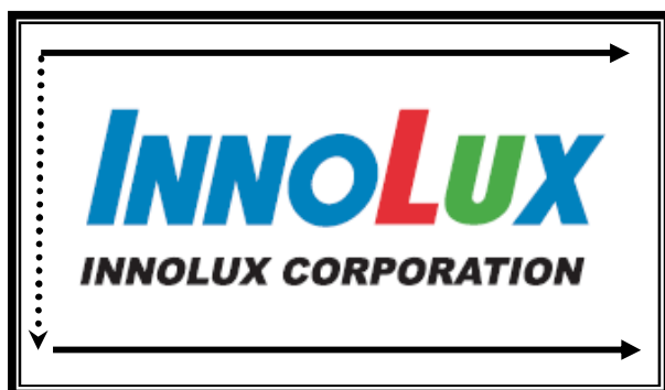
Fig. 1 Normal scan ( pin 4, LR/UD = High or NC )
