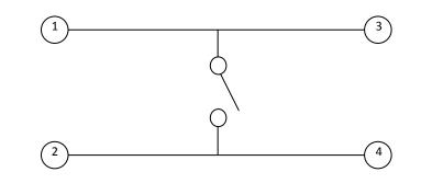
**Dimensions:** CHECKED REVISION DATE (YYYY-MM-DD) GENERAL TOLERANCE PROJECTION METHOD ELin 003.002 2021-01-07 DIN ISO 2768-1m Properties Value Unit DESCRIPTION Height Н 5 mm **WS-TATV THT Tact Switch** ØD 3.5 Diameter mm Würth Elektronik eiSos GmbH & Co. KG ORDER CODE EMC & Inductive Solutions Max-Eyth-Str. 1 430156050736 74638 Waldenburg Germany SIZE/TYPE STATUS Tel. +49 (0) 79 42 945 - 0 www.we-online.com BUSINESS UNIT PAGE WÜRTH ELEKTRONIK 6 x 6 mm eiCan Valid 1/8 eiSos@we-online.com
