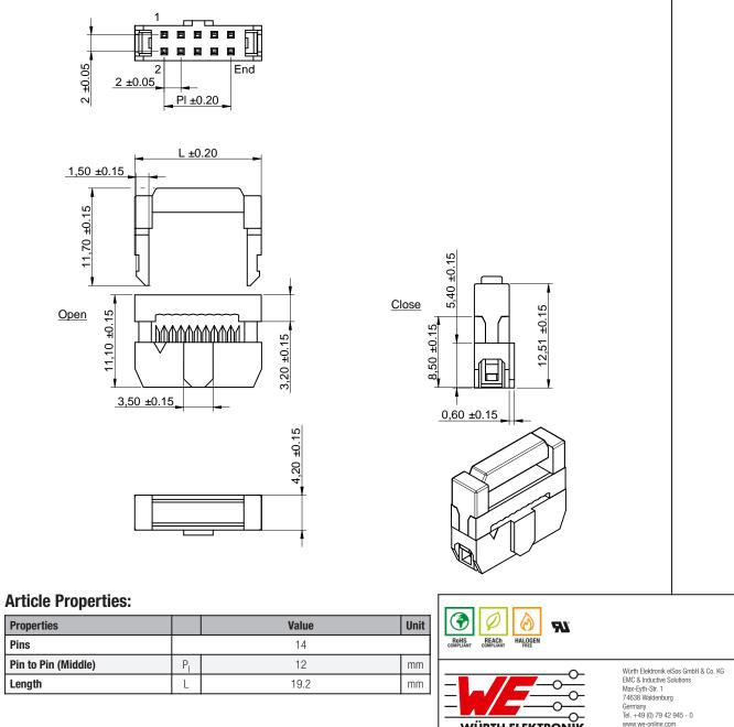
CHECKED DATE (YYYY-MM-DD) GENERAL TOLERANCE PROJECTION METHOD REVISION Ð ATo 001.001 2019-12-05 DIN ISO 2768-1m DESCRIPTION **WR-BHD Female IDC Connector** ORDER CODE 62501423021 SIZE/TYPE STATUS BUSINESS UNIT PAGE with Strain Relief, 2.00 mm eiCan Valid 1/6
