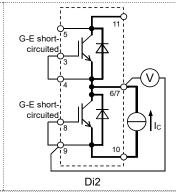
V<sub>CEsat</sub> characteristics test circuit
