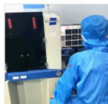
Trioptics-Pro9 MTF Lens test parsing /EF
