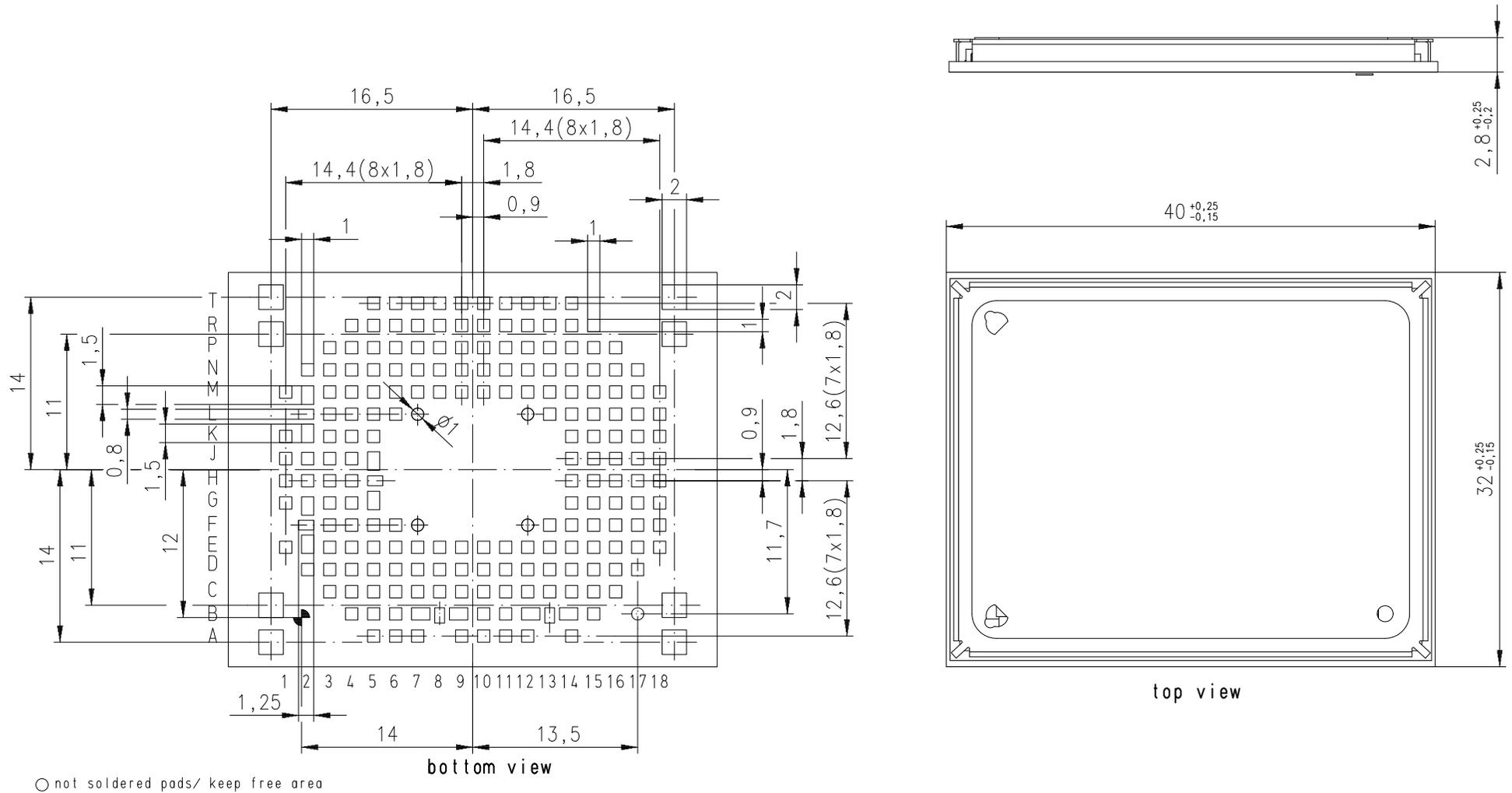
Figure 32: Dimensions of PLAS9-W (all dimensions in mm)
