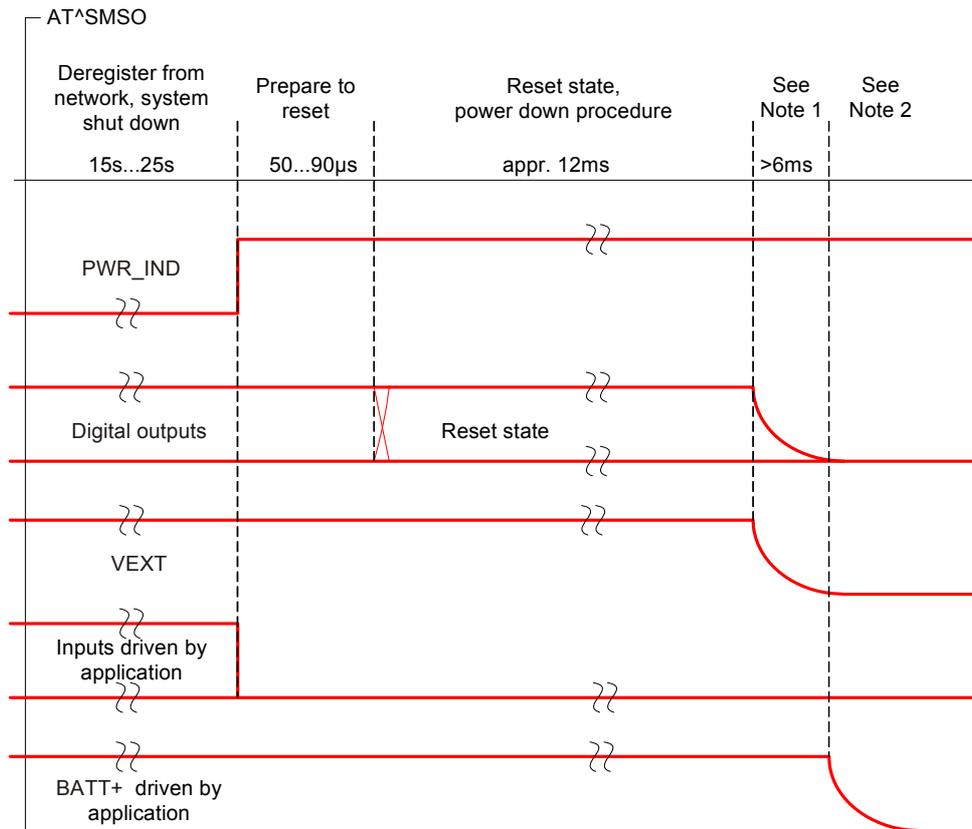
Figure 21: Signal states during turn-off procedure
