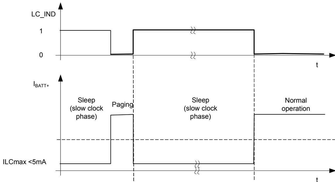
**Figure 10:** Low current indication timing
