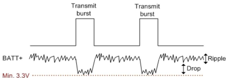
Figure 29: Power supply limits during transmit burst
