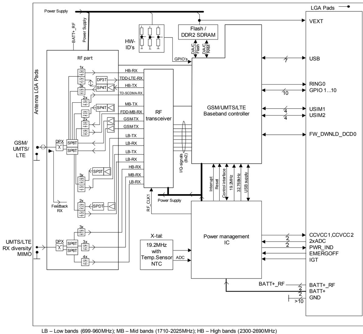
Figure 2: PLAS9-W block diagram
