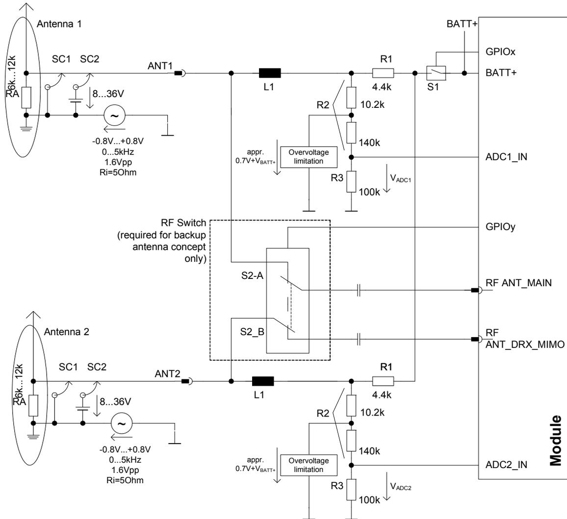
Figure 16: Basic layout sample for antenna detection
