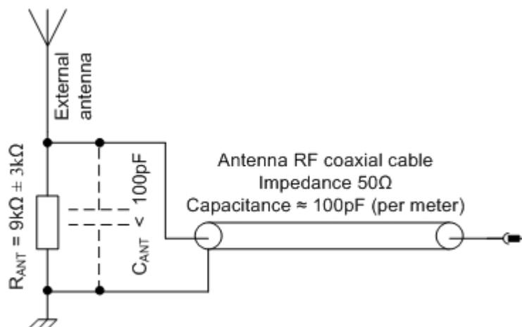
Figure 15: Resistor measurement used for antenna detection
