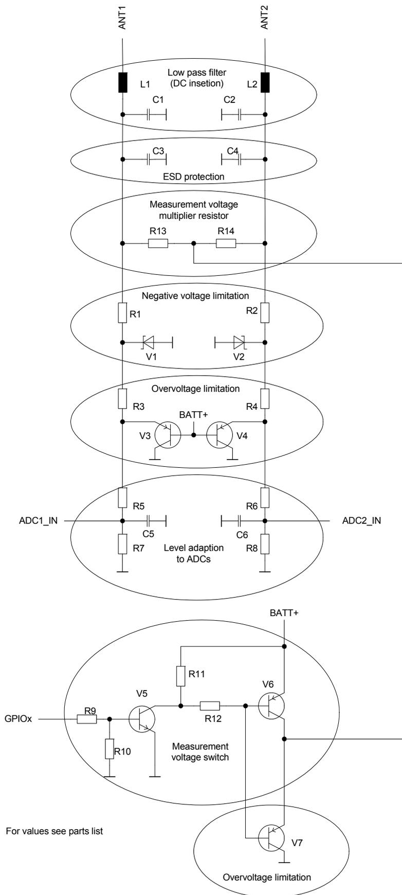
Figure 19: Antenna detection circuit sample - schematic
