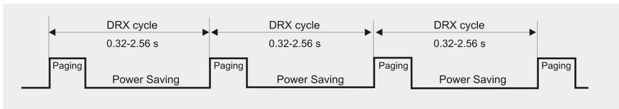
**Figure 27:** Power saving and paging in LTE networks
