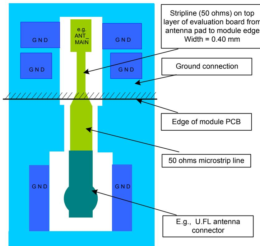
Figure 14: Routing to application's RF connector
