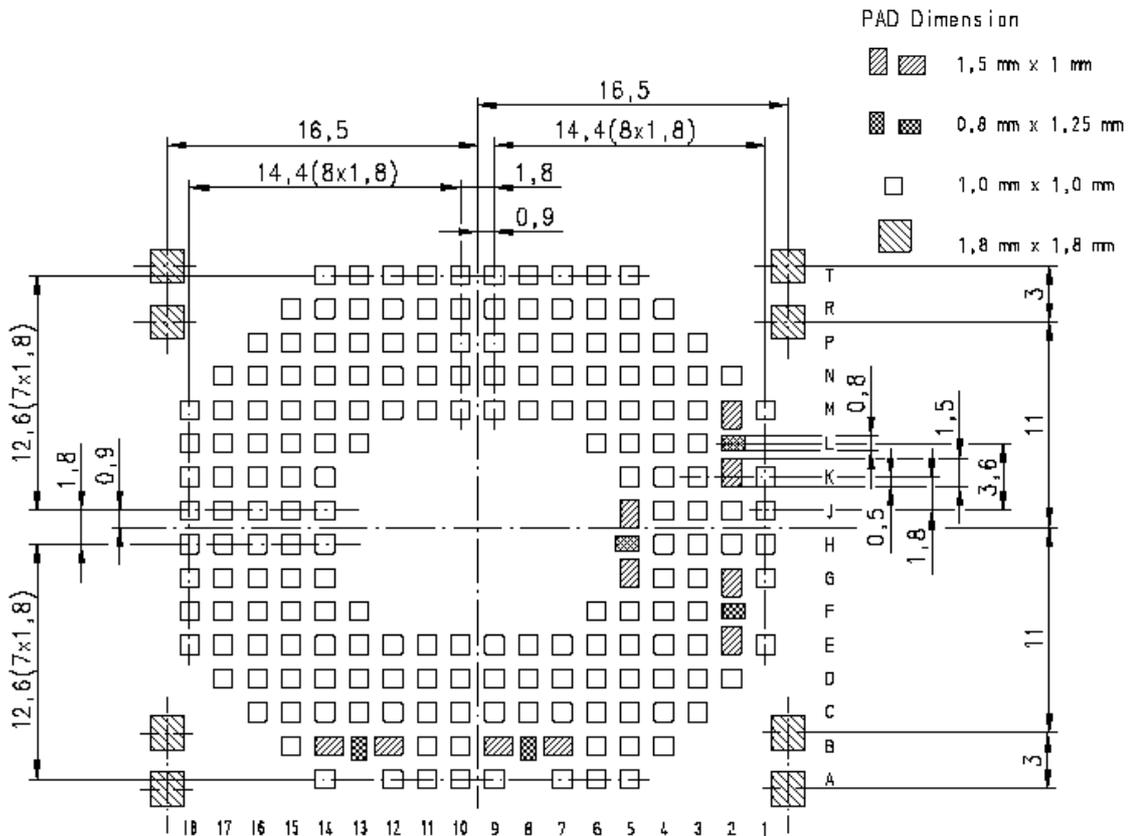
Figure 34: Recommended design for 110 micron thick stencil (top layer)
