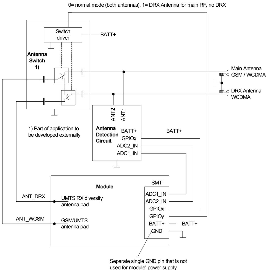
**Figure 18:** Antenna detection circuit sample - overview
