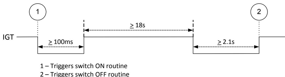
**Figure 22:** Timing of IGT if used as ON/OFF switch
