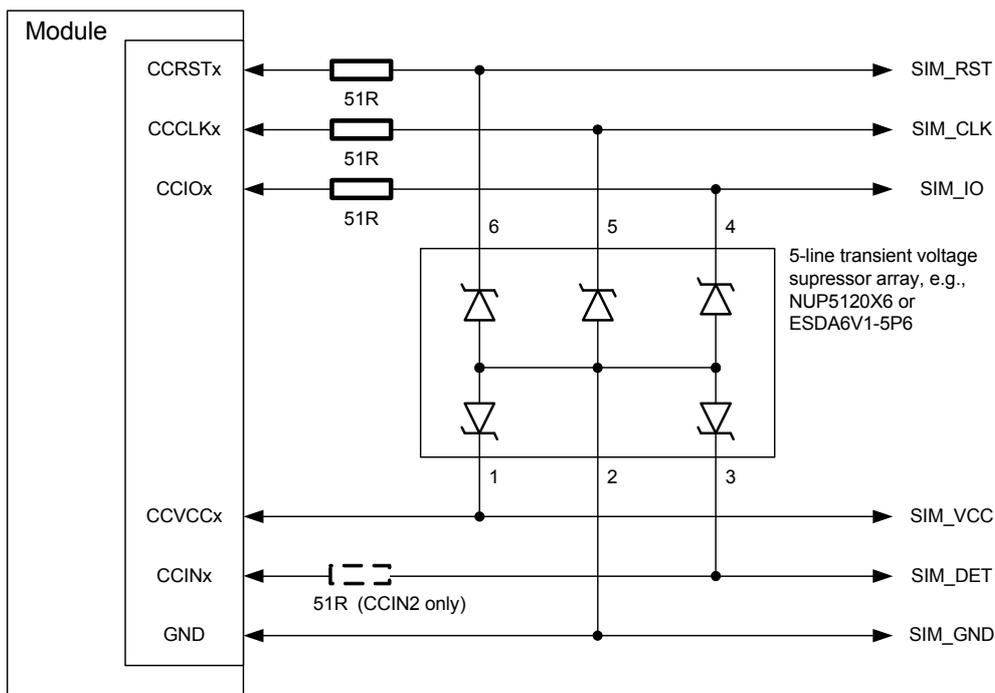
Figure 8: SIM interfaces - enhanced ESD protection
