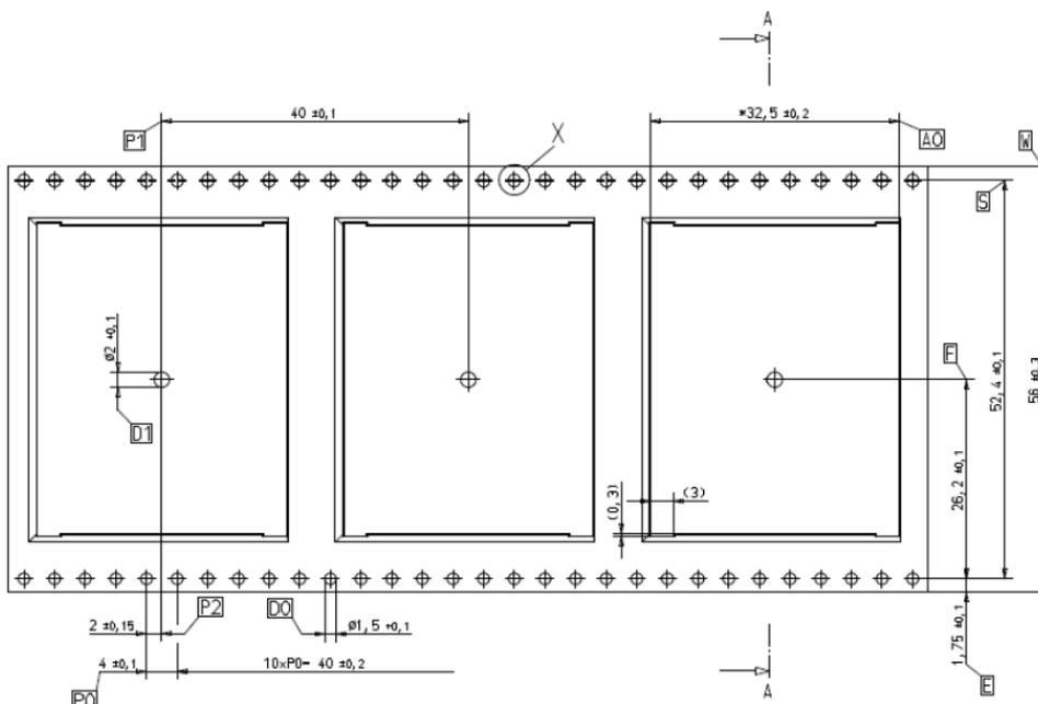
Figure 36: Carrier tape dimensions
