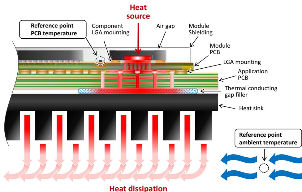
Figure 30: Board and ambient temperature differences
