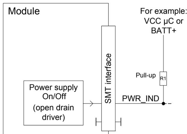
Figure 9: PWR\_IND signal
