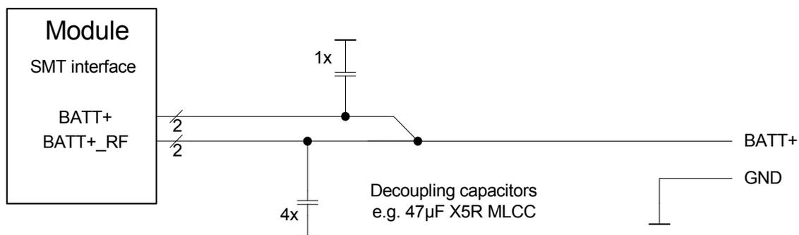
**Figure 28:** Decoupling capacitor(s) for BATT+
