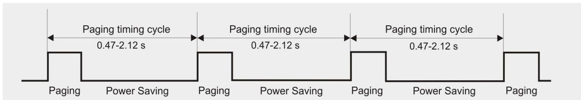
**Figure 25:** Power saving and paging in GSM networks
