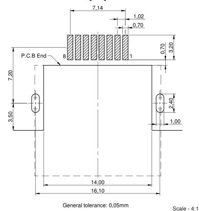
GENERAL TOLERANCE PROJECTION METHOD Würth Elektronik eiSos GmbH & Co. KG CREATED CHECKED **EMC & Inductive Solutions** DaSc CLe DIN ISO 2768-1m Max-Eyth-Str. 1 74638 Waldenburg **WR-MJ Modular Jack Tab Up** Tel. +49 (0) 79 42 945 - 0 Middle mounted Shielded SMT ORDER CODE www.we-online.com 634108150321 **8P8C** eiSos@we-online.com DATE (YYYY-MM-DD) REVISION STATUS BUSINESS UNIT PAGE 001.000 Valid 2018-08-07 1/5 **WÜRTH ELEKTRONIK**
