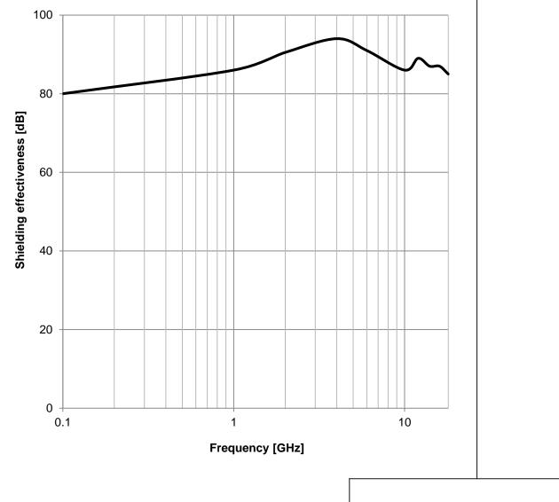
CHECKED REVISION DATE (YYYY-MM-DD) GENERAL TOLERANCE PROJECTION METHOD JoV 005.002 2019-01-01 DIN ISO 2768-1m DESCRIPTION **WE-LT Conductive Shielding** Würth Elektronik eiSos GmbH & Co. KG Gasket ORDER CODE EMC & Inductive Solutions Max-Eyth-Str. 1 38008027 74638 Waldenburg Germany SIZE/TYPE STATUS Tel. +49 (0) 79 42 945 - 0 www.we-online.com BUSINESS UNIT PAGE WÜRTH ELEKTRONIK 2/3 Knife-Edge eiSos Valid eiSos@we-online.com
