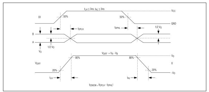
Figure 3. Driver Propagation Delays
