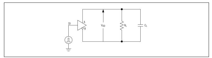
Figure 2. Driver Timing Test Circuit
