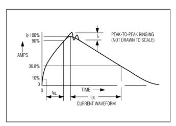
Figure 11. Human Body Current Waveform
