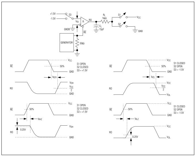
Figure 8. Receiver Enable and Disable Times
