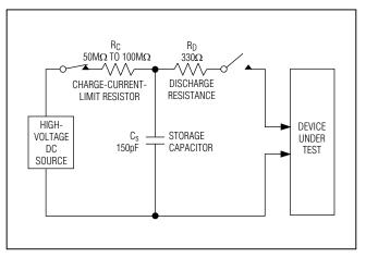
Figure 12. IEC 61000-4-2 ESD Test Model
