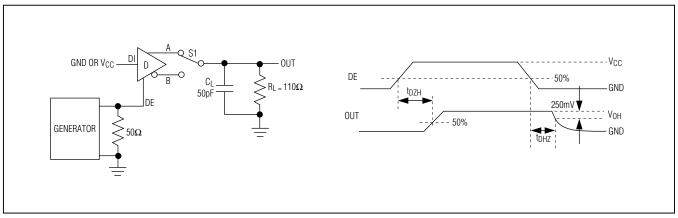
Figure 4. Driver Enable and Disable Times (t<sub>DHZ</sub>, t<sub>DZH</sub>)
