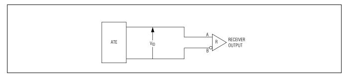
Figure 6. Receiver Propagation Delay Test Circuit
