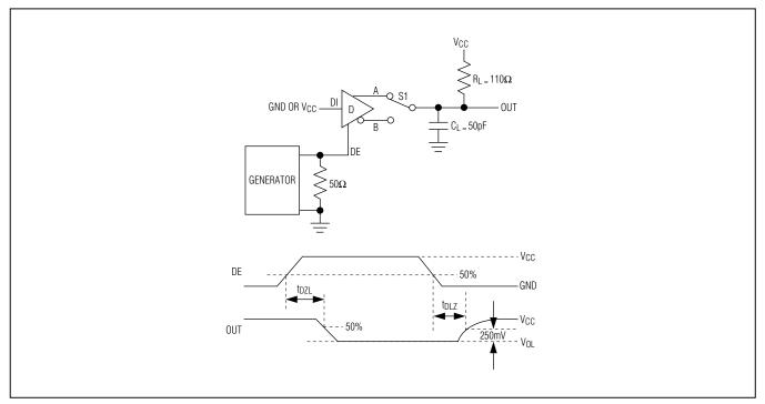
Figure 5. Driver Enable and Disable Times (t<sub>DZL</sub>, t<sub>DLZ</sub>)
