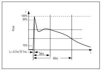
Figure 13. IEC 61000-4-2 ESD Generator Current Waveform
