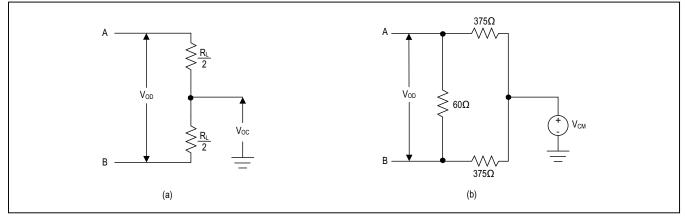
Figure 1. Driver DC Test Load
