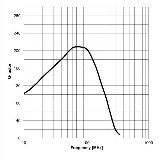
GENERAL TOLERANCE Würth Elektronik eiSos GmbH & Co. KG CREATED CHECKED **EMC & Inductive Solutions** KaS JoMa DIN ISO 2768-1m Max-Eyth-Str. 1 74638 Waldenburg **WE-ACHC High current air coil** Tel. +49 (0) 79 42 945 - 0 ORDER CODE www.we-online.com 7449152111 eiSos@we-online.com DATE (YYYY-MM-DD) BUSINESS UNIT REVISION PAGE 001.000 2017-01-26 2/6 1212 Valid **WÜRTH ELEKTRONİK**
