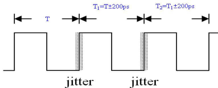
Note (4) The SSCG (Spread spectrum clock generator) is defined as below figures.
