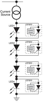
Note: The interaction between the Bourns® LSP device and the power supply for the LED series string dictates the power supply architecture. Proper care must be taken in the design of the power supply architecture to ensure that the Bourns® LSP devices operate as intended and the design maintains integrity.
