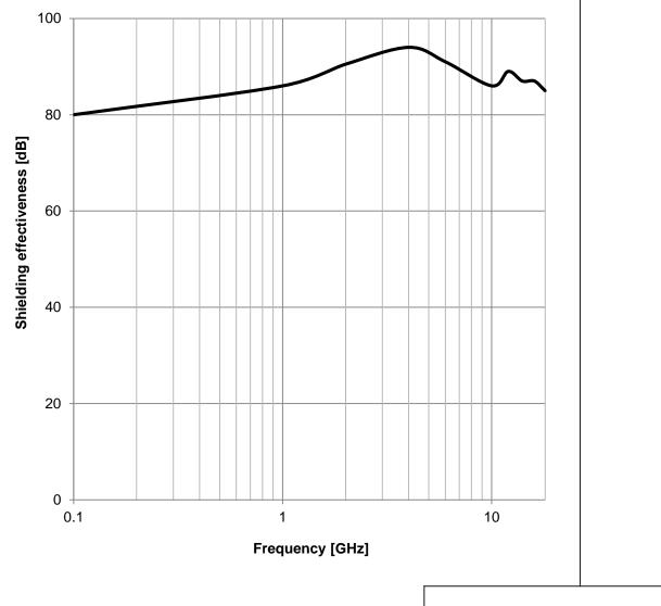
CHECKED REVISION DATE (YYYY-MM-DD) GENERAL TOLERANCE PROJECTION METHOD ViMa 004.003 2020-03-06 DIN ISO 2768-1m DESCRIPTION **WE-LT Conductive Shielding** Würth Elektronik eiSos GmbH & Co. KG Gasket ORDER CODE EMC & Inductive Solutions Max-Eyth-Str. 1 3020905 74638 Waldenburg Germany SIZE/TYPE STATUS Tel. +49 (0) 79 42 945 - 0 www.we-online.com BUSINESS UNIT PAGE WÜRTH ELEKTRONIK 2/3 eiSos Valid Square eiSos@we-online.com
