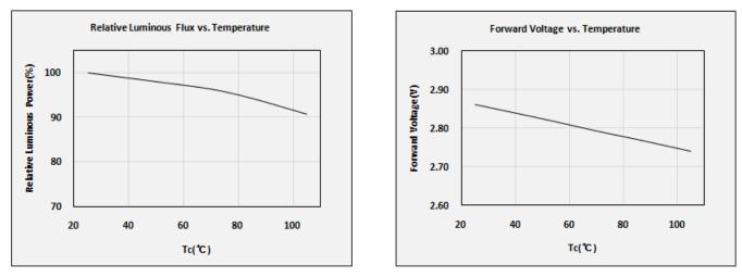
e) Derating Curve and Beam Angle Characteristics  $(I_F = 350 \text{ mA})$
