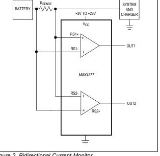
Figure 2. Bidirectional Current Monitor
