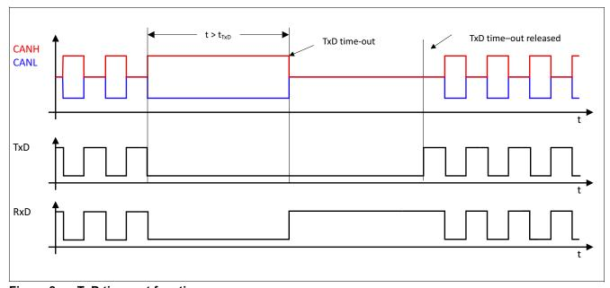
Figure 8 TxD time-out function
