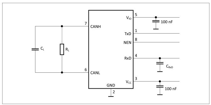
Figure 10 Test circuits for dynamic characteristics
