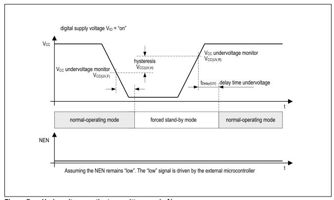
Figure 7 Undervoltage on the transmitter supply  $V_{\rm CC}$
