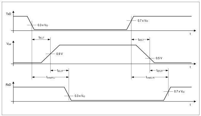
Figure 11 Timing diagrams for dynamic characteristics
