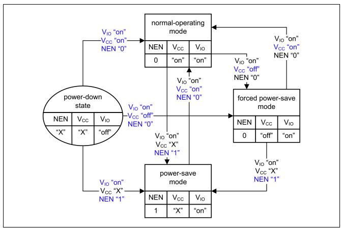
Figure 5 Power-up and undervoltage
