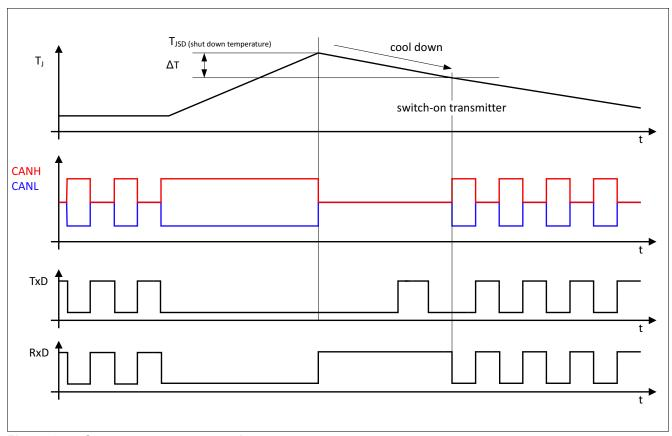
Figure 9 Overtemperature protection
