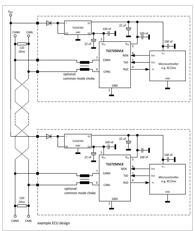
Figure 13 Application circuit
