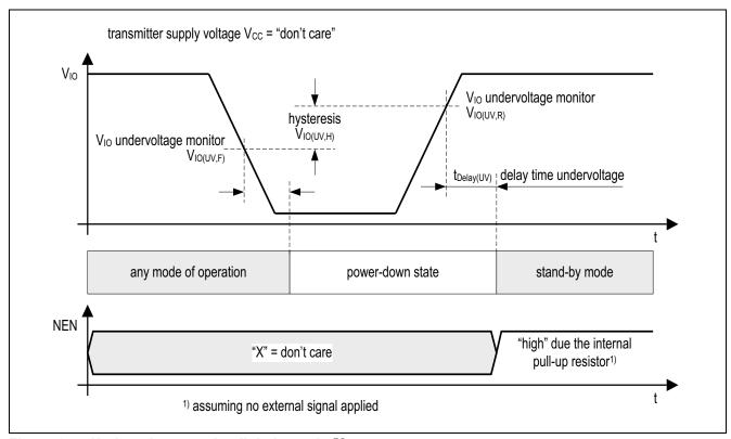
Figure 6 Undervoltage on the digital supply  $V_{\rm IO}$
