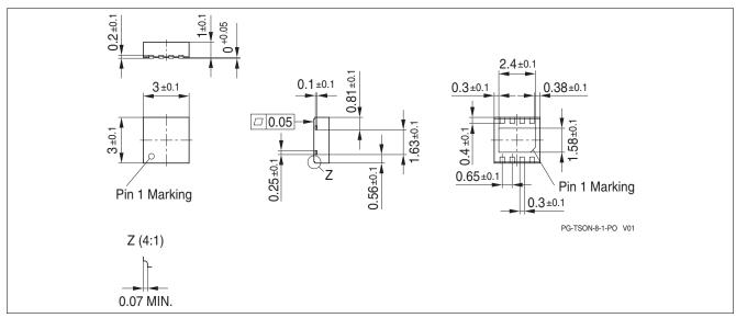
Figure 16 PG-TSON-8 (Plastic Thin Small Outline Nonleaded PG-TSON-8-1)
