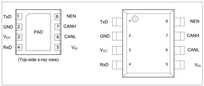
Figure 2 Pin configuration
