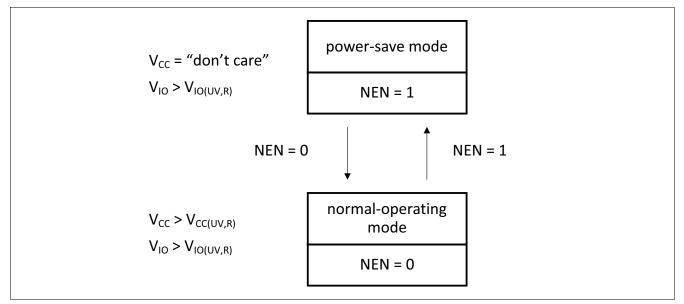
Figure 4 Mode state diagram
