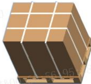
Place out box and wrap film around the boxes. Pack with 4 packing belts.
