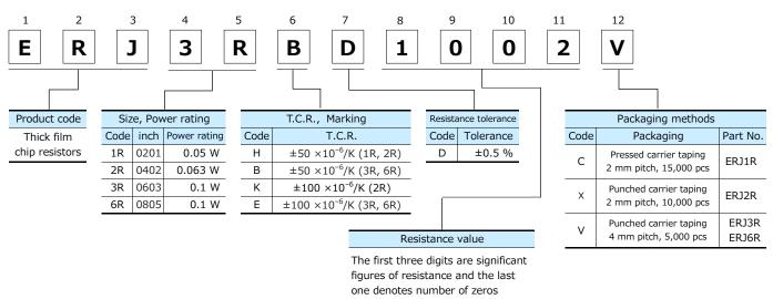
following. Example :  $1002 \rightarrow 10 \text{ K}\Omega$  • ERJXGN, 1GN, 2RC, 2RK, 3EK, 6EN, 8EN, 14N, 12N, 12S, 1TN series : ±1 %
