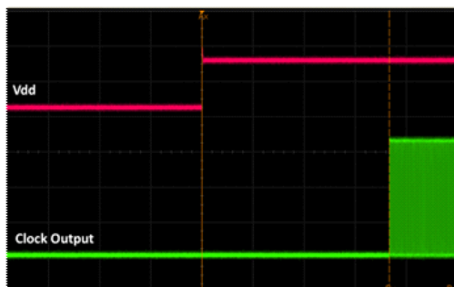
Figure 17. Startup Waveform vs. Vdd
