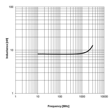
DESCRIPTION Projection **WE-CAIR Air coil** Würth Elektronik eiSos GmbH & Co. KG EMC & Inductive Solutions Max-Eyth-Str. 1 Order.- No. 74638 Waldenburg COMPLIANT SIZE Germany Tel. +49 (0) 79 42 945 - 0 744913080 www.we-online.com A4 SSt 1.0 2015-02-12 HBH eiSos@we-online.com REV BY Size: 3136 DATE CHECKED
