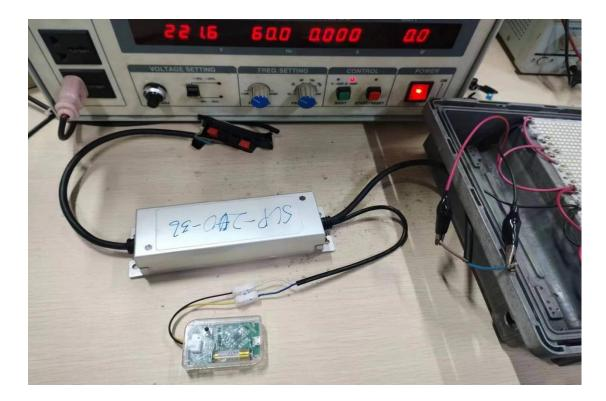
PS: The color of the wires in different products may be different, please see the products label. But there is one thing in common: The black wire connect to DIM-. and The Yellow / blue wire connect to DIM + . The most of the products is DIM- is color pink, and the DIM + is color purple
