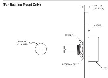
Panel thickness and hole diameters are recommended for best fit. However, customers may adjust the dimensions to suit their specific application.
