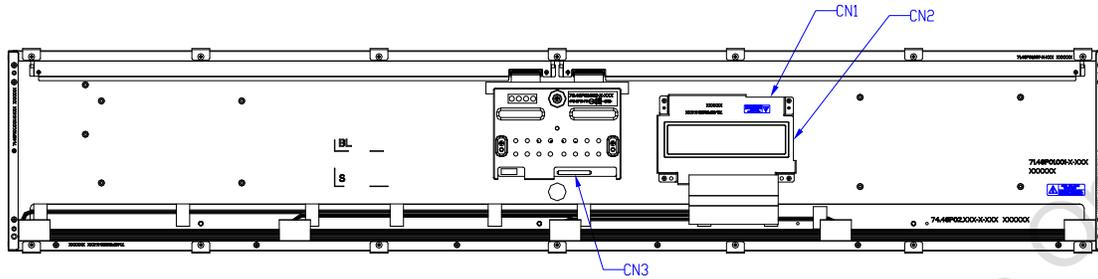
LED DB connector (CN1): No connection (for AUO internal use only)
