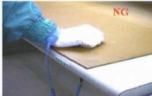
12.4 Please do not bend the film near the substrate glass. (this could cause film peeling and COF damage) and the peeling strength about 600g/cm, the bending <20times and the bending radius : $R > 0.8\text{mm}$
