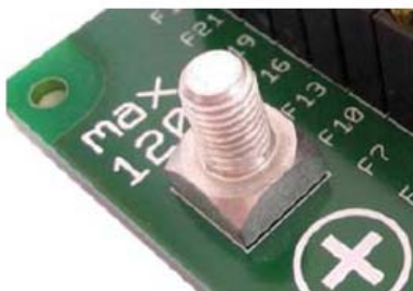
DC power connection up to 120 A
