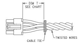
The "T" dimension defines a "free" length of wire, or a length of wire that is not subject to significant bias by external factors such as a wire tie, wire twisting, or other means of bending or deforming of the wires that repositions them from their natural relaxed state or location where they enter the housing. Wires are to be dressed in such a manner to allow the terminals to float freely in the pocket.
