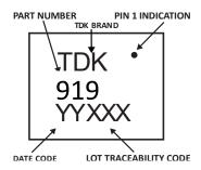
Figure 18. Package Marking Specification (Top View)
