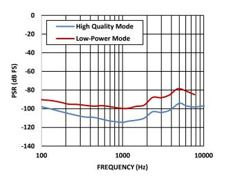
Figure 8. Power Supply Rejection (PSR) vs. Frequency
