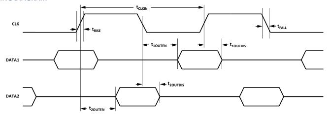
Figure 1. Pulse Density Modulated Output Timing
