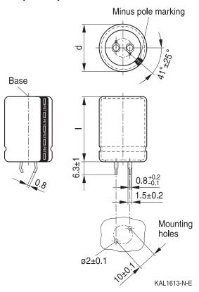
Snap-in terminals, length  $(6.3 \pm 1)$  mm. Also available in a shorter version with a length of (4.5 - 1) mm. PET insulation is marked with "PET" on the sleeve. Safety vent on the base or on the case wall.
