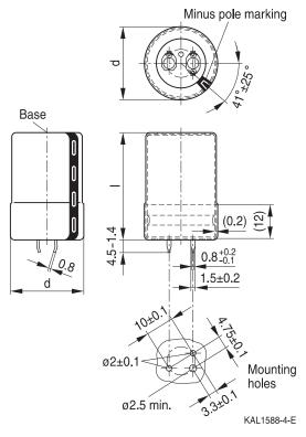
Snap-in capacitors are also available with 3 terminals (length (4.5-1.4) mm). PET insulation cap is positioned under the insulation sleeve. Safety vent on the base or on the case wall.
