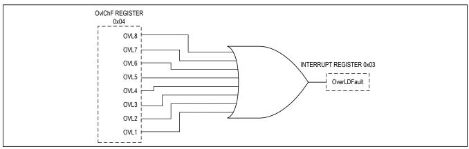
Figure 7. Overload Interrupt Diagnostic Scheme
