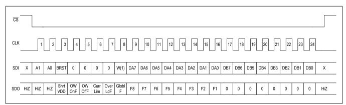
Figure 12. Addressed SPI Single Cycle Write Command
