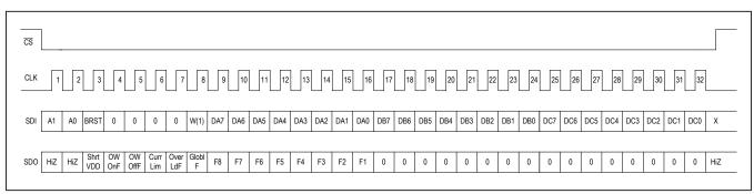
Figure 13. Addressed SPI Three Bytes Burst Write Command
