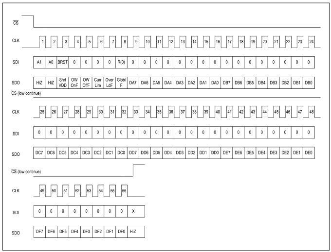
Figure 15. Addressed SPI Six Bytes Burst Read Command
