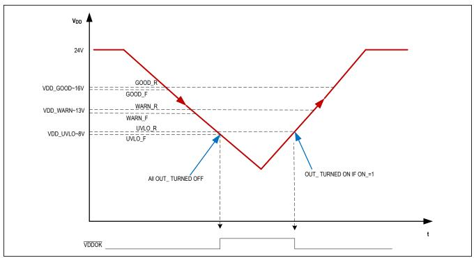
Figure 3.  $V_{DD}$  Monitoring with VDDOnThr = 0
