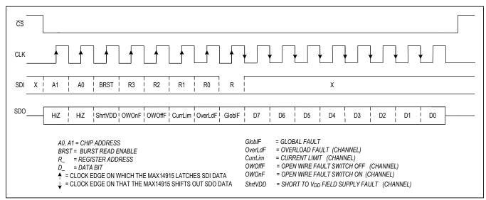
Figure 10. Addressed SPI Single Read Command
