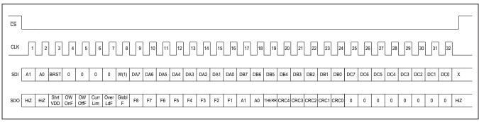
Figure 14. Addressed SPI Two Bytes Burst Write Command with CRC
