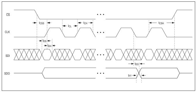
Figure 1. SPI Timing Diagram.
