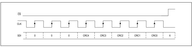
Figure 19. FCS Byte Expected from the SPI Master
