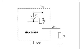
Figure 22. Inductive Load Clamping Scheme
