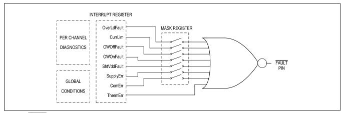
Figure 8. FAULT Signaling Scheme
