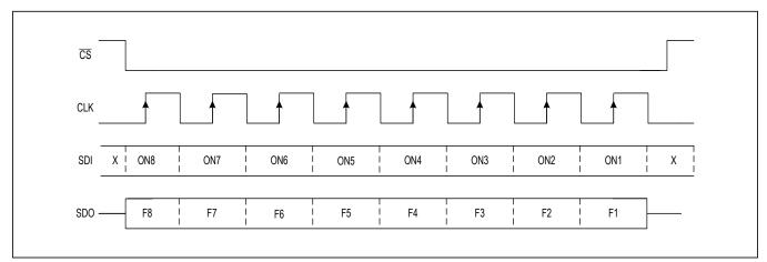
Figure 18. Single Daisy-Chain SPI Command
