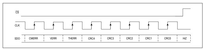
Figure 21. FCS Byte Sent by the MAX14915 to SPI Master in Daisy-Chain Mode
