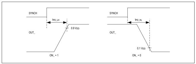
Figure 2. Propagation Delay Timing Characteristics
