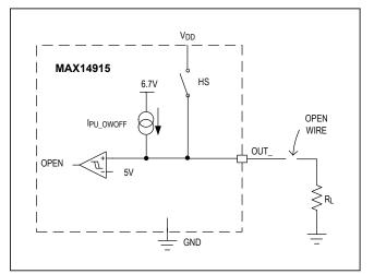
Figure 5. Open Wire Detection Scheme
