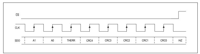
Figure 20. FCS Byte Sent by the MAX14915 to SPI Master (SPI Addressed Mode)
