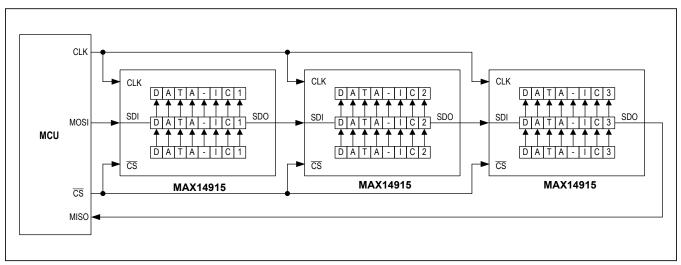
Figure 17. Daisy-Chaining Diagram of Three MAX14915
