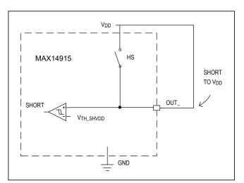
Figure 6. Short to V<sub>DD</sub> Detection Scheme
