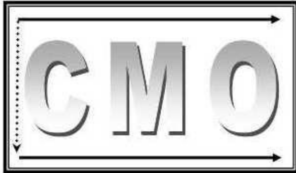
Fig. 1 Normal scan ( pin 4, DPS = Low or NC)
