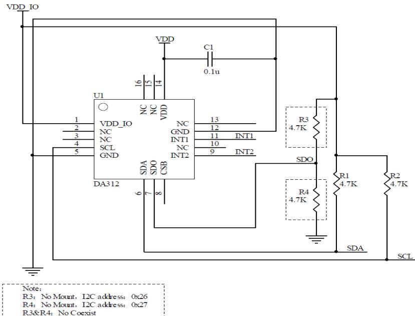
**Figure 12 da312 I2C electrical connect**
