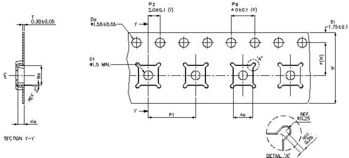
Figure 15 Tape and reel dimension in mm
