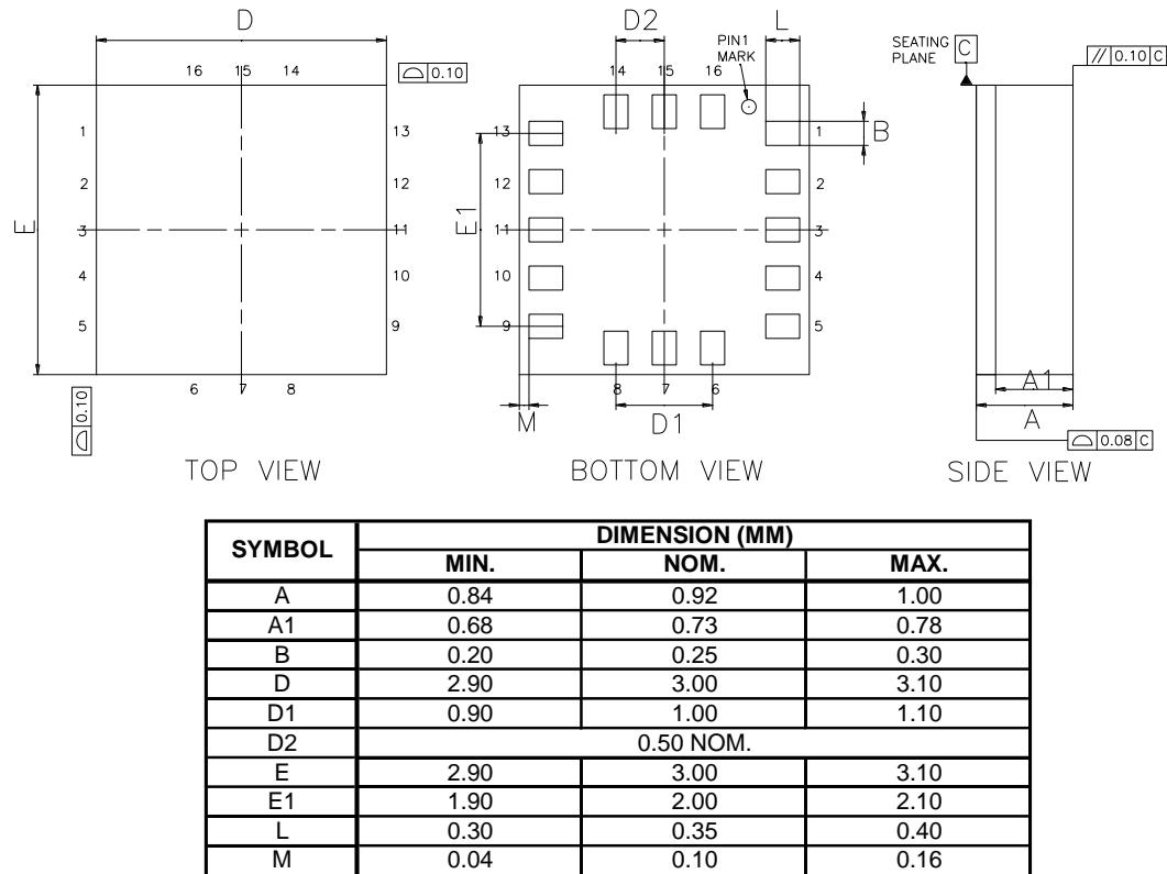
Figure 14 12 Pin LGA Mechanical data and package dimensions
