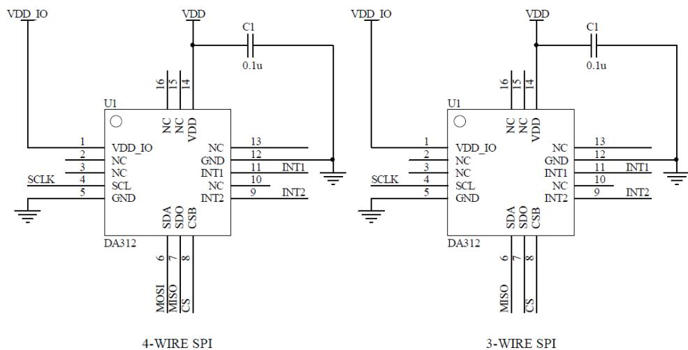
**Figure 13 da312 SPI electrical connect**
