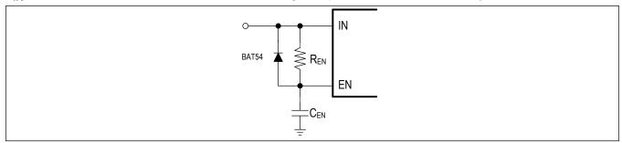
Figure 1. RC Circuit at EN
