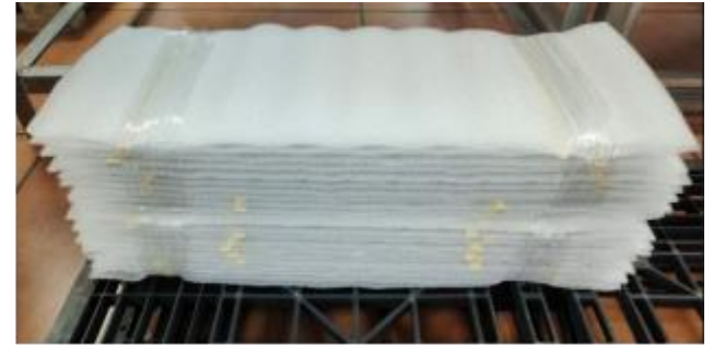
3. A total of 14 panels are packed in one bundle (one layer of foam is added on the top layer), and wrapped with winding. 4. Each box contains 2 bundles, and the quantity of each box is 420PCS; the film is wound and fixed;
