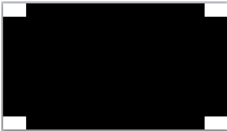
Black center measurement is made with 10% linear boxes in corners ; L_k (1/10 size of H and V of display)
