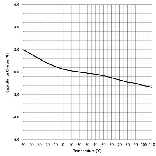
Test Equipment: E4991A or equivalent
