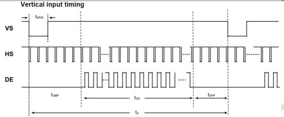
Figure 5.2.2 Vertical input timing
