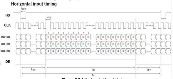
Figure 5.2.1 Horizontal input timing
