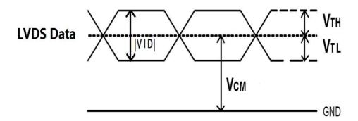
Figure 4.1 LVDS DC characteristics
