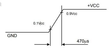
Figure 4.2 Inrush current test condition
