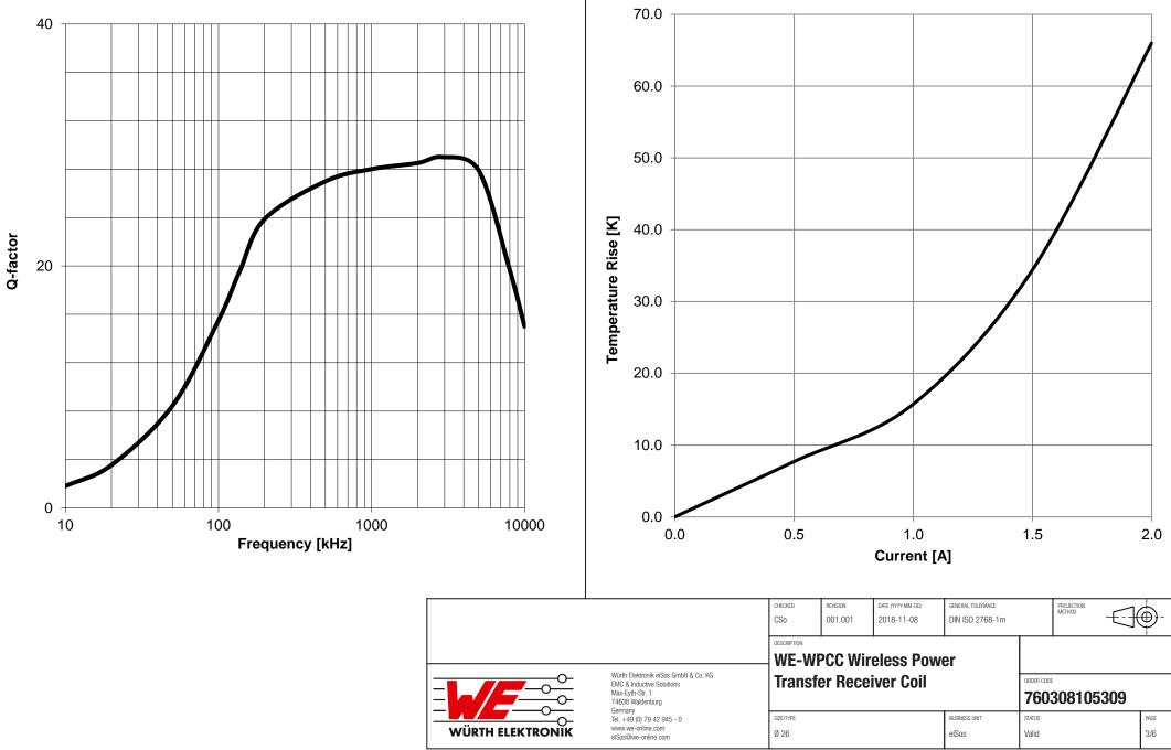
**Typical Temperature Rise vs. Current Characteristics:**
