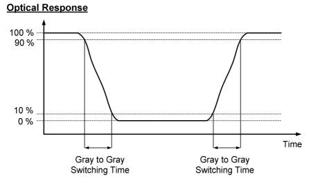
The driving signal means the signal of gray level 0, 31, 63, 95, 127, 159, 191, 223 and 255.
