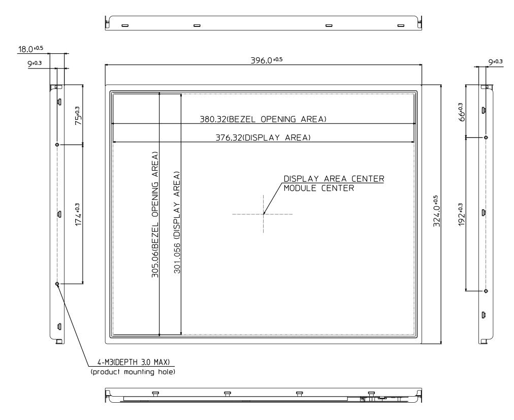
Note1: The torque for product mounting screws must never exceed  $0.67N \cdot m$ . And the length of product mounting screws from surface of plate (product side) must be  $\leq 3.0$  mm.
