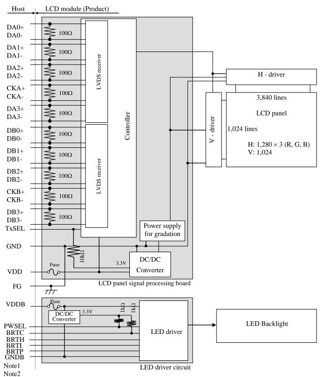
Note1: Relations between GND (Signal ground), GNDB (LED driver ground) and FG (Frame ground) in the LCD module are as follow.
