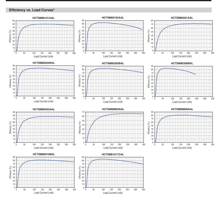
\*Measured with circuit in Typical Application, 5 VDC input, 0-350 mA DC load,  $T_a = 20 \, ^{\circ}\mathrm{C}$
