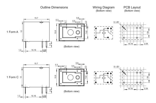
Remark: 1) The pin dimension of the product outline drawing is the size before tinning(it will become larger after tinning), and the mounting hole size is the recommended design size of the PCB board hole. The specific PCB board hole design size can be mapped and adjusted according to the actual product.
