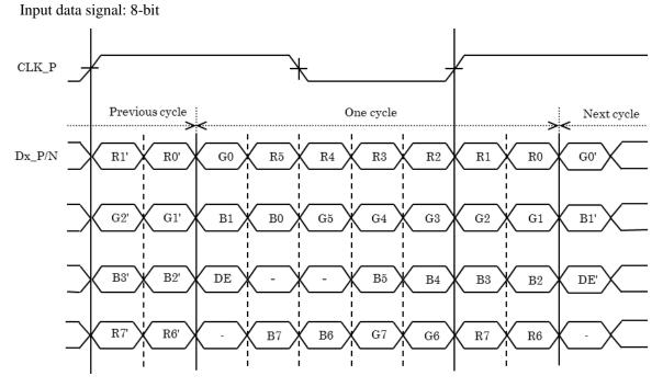
Note1: LSB (Least Significant Bit) – R0, G0, B0 MSB (Most Significant Bit) – R7, G7, B7
