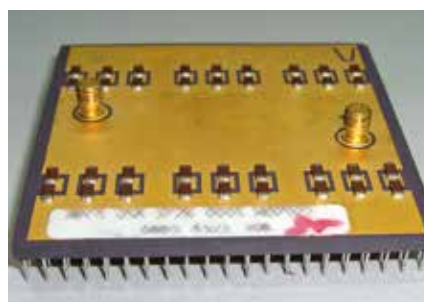
High-mass ceramic Pin Grid Array
