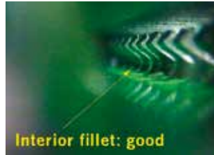
PLCC – interior fillet inspection
