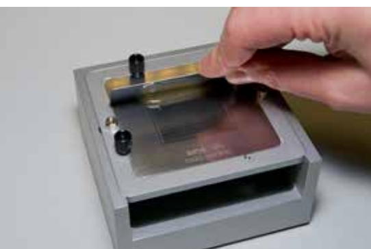
Flux deposition in the dip stencil
