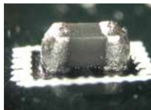
0402: bulbous solder joint
