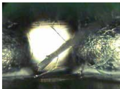
BGA: contamination (fibre)
