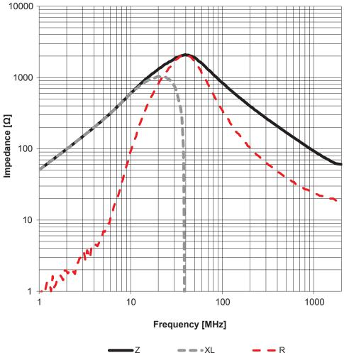
Test Equipment: E4991A or equivalent
