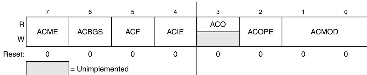
Figure 9-3. ACMP Status and Control Register
