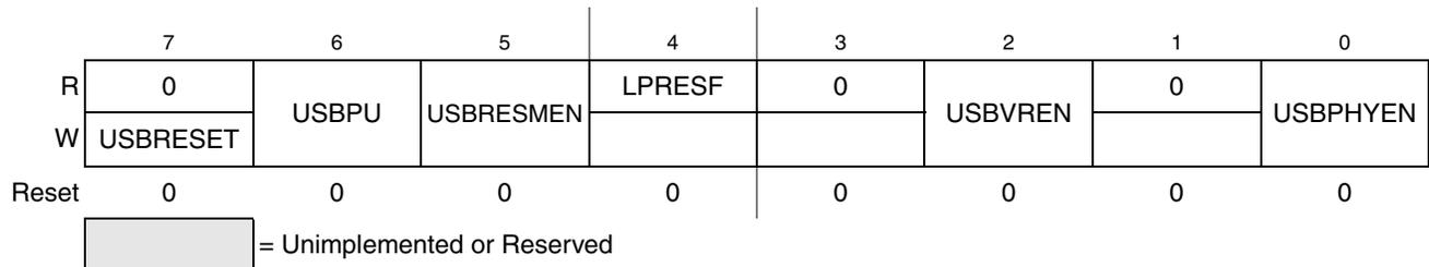
**Figure 17-3. USB Transceiver and Regulator Control Register 0 (USBCTL0)**
