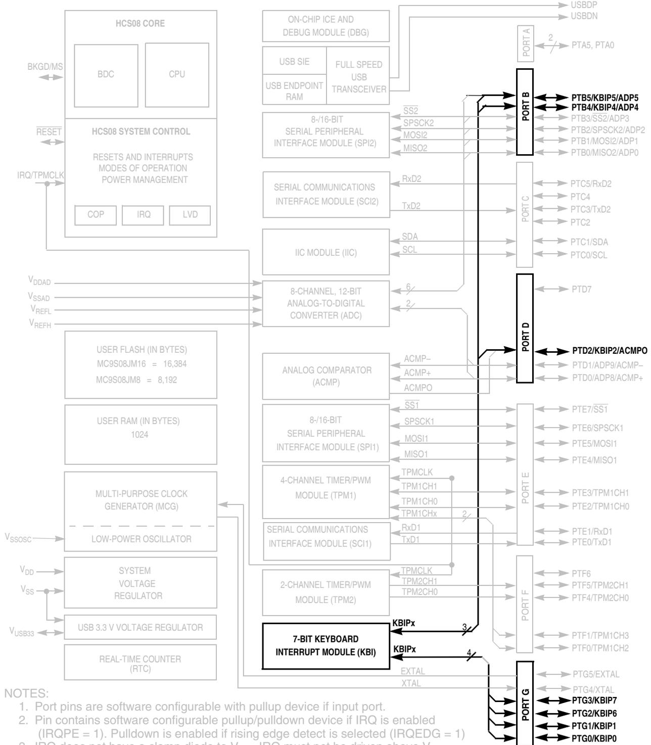
Figure 8-1. MC9S08JM16 Series Block Diagram Highlighting KBI Block and Pins
