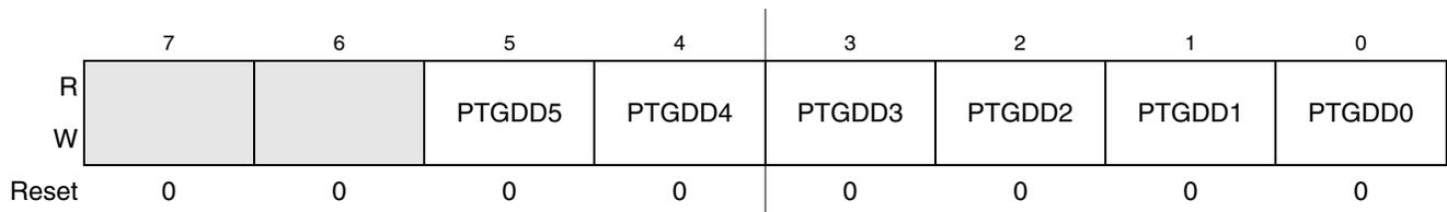
Figure 6-33. Data Direction for Port G (PTGDD)
