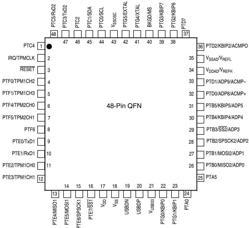
Figure 2-1. MC9S08JM16 Series in 48-Pin QFN Package
