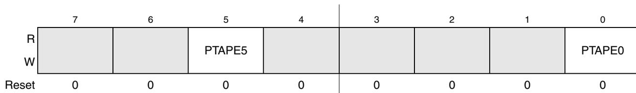
Figure 6-4. Internal Pullup Enable for Port A (PTAPE)
