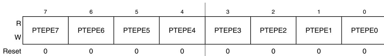
Figure 6-24. Internal Pullup Enable for Port E (PTEPE)
