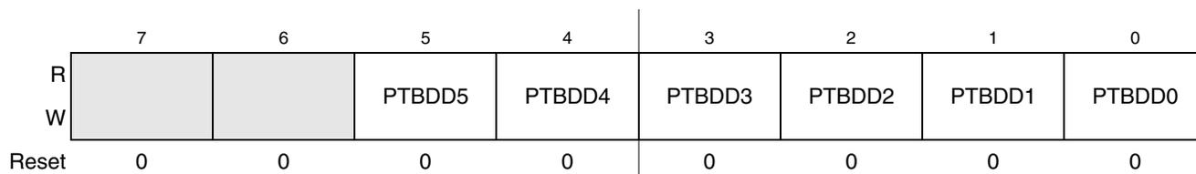
**Figure 6-8. Data Direction for Port B (PTBDD)**
