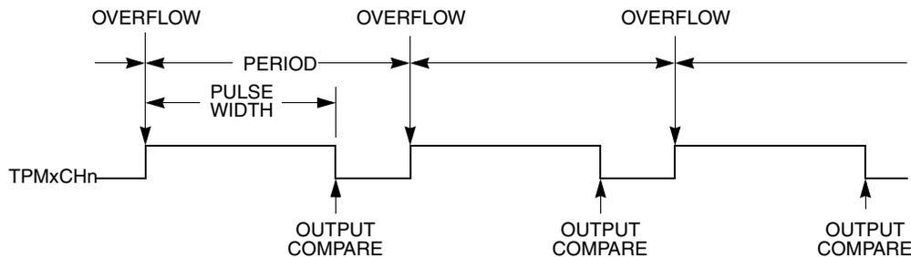
Figure 16-15. PWM Period and Pulse Width (ELSnA=0)
