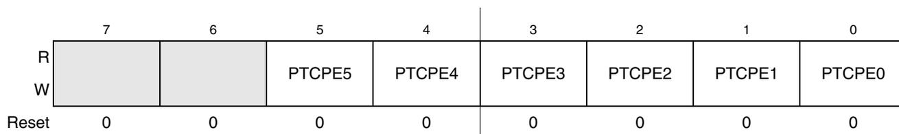
Figure 6-14. Internal Pullup Enable for Port C (PTCPE)
