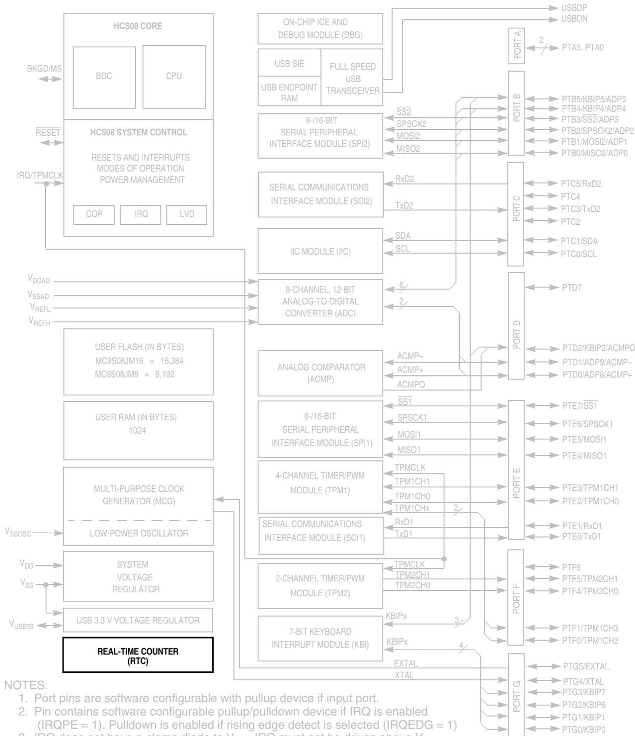
Figure 13-1. MC9S08JM16 Series Block Diagram Highlighting RTC Block
