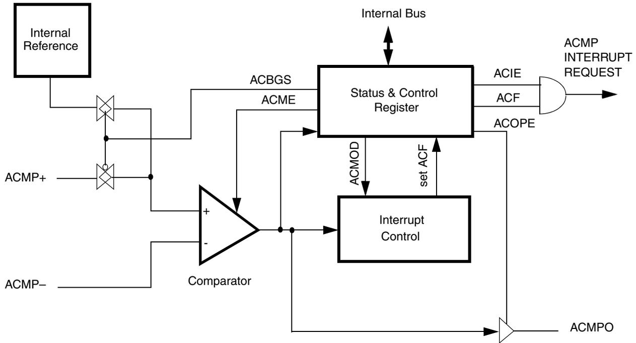
Figure 9-2. Analog Comparator 5V (ACMP5) Block Diagram
