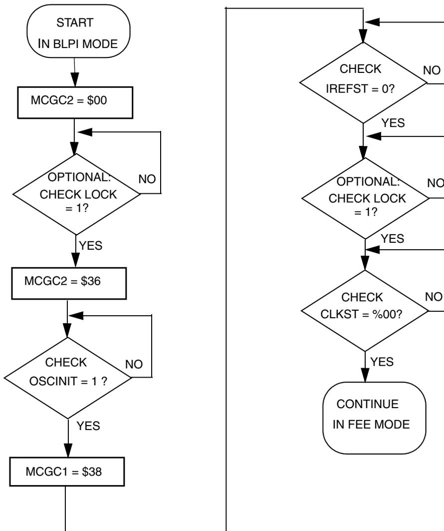
Figure 12-11. Flowchart of BLPI to FEE Mode Transition using a 4 MHz Crystal
