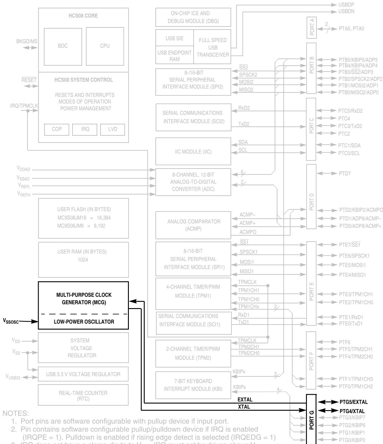
Figure 12-1. MC9S08JM16 Series Block Diagram Highlighting MCG Block and Pins
