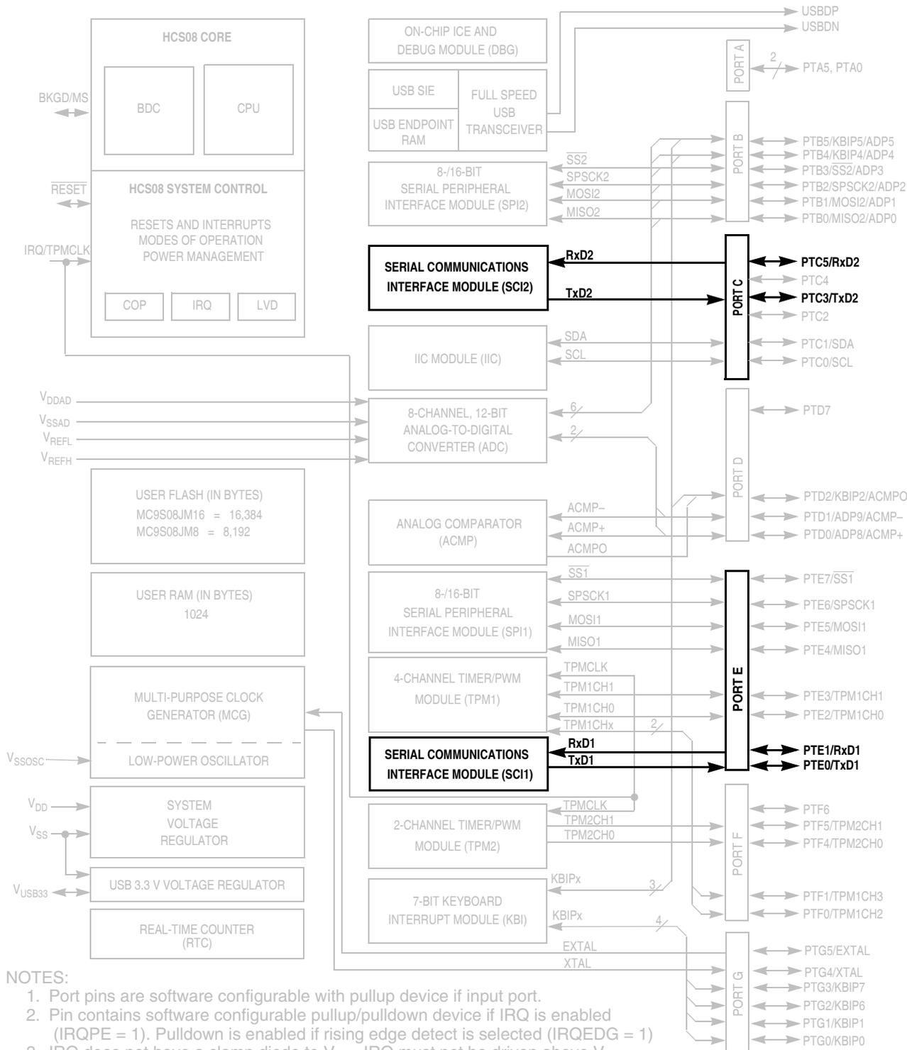
Figure 14-1. MC9S08JM16 Series Block Diagram Highlighting the SCI Blocks and Pins
