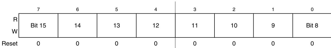
**Figure 16-13. TPM Channel Value Register High (TPMxCnVH)**
