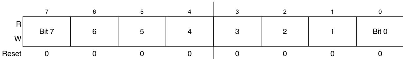
**Figure 16-11. TPM Counter Modulo Register Low (TPMxMODL)**
