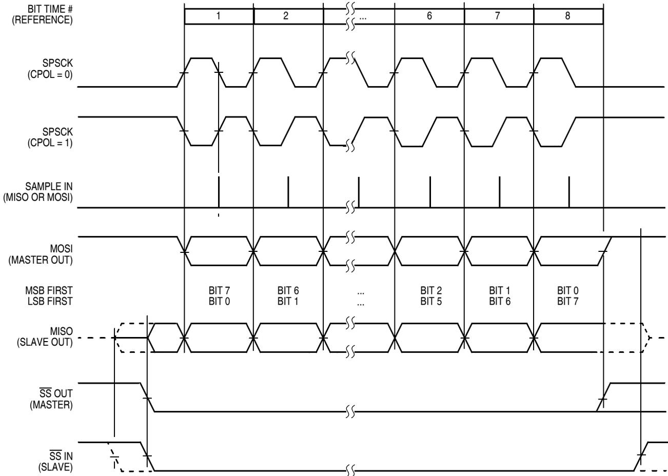
**Figure 15-13. SPI Clock Formats (CPHA = 1)**
