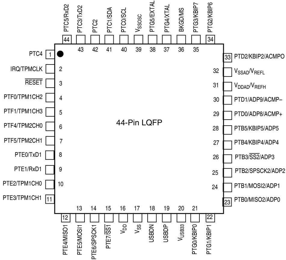
Figure 2-2. MC9S08JM16 Series in 44-Pin LQFP Package
