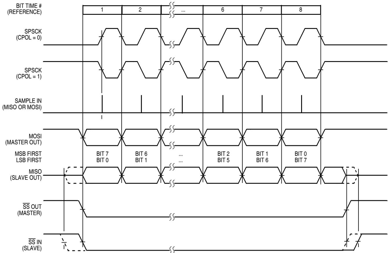
Figure 15-14. SPI Clock Formats (CPHA = 0)
