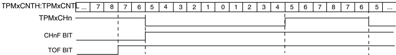
**Figure 16-6. Low-True Pulse of a Center-Aligned PWM**
