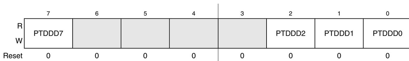
Figure 6-18. Data Direction for Port D (PTDDD)
