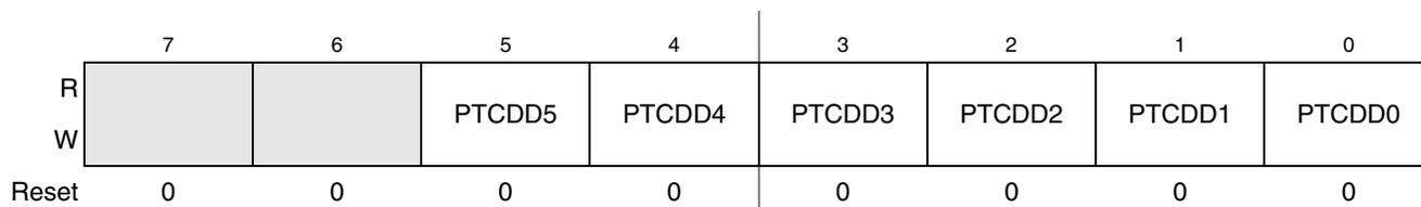
Figure 6-13. Data Direction for Port C (PTCDD)
