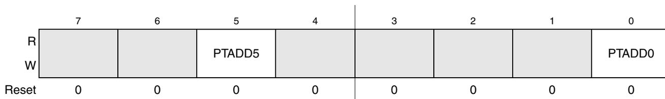
Figure 6-3. Data Direction for Port A Register (PTADD)
