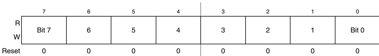
**Figure 16-14. TPM Channel Value Register Low (TPMxCnVL)**
