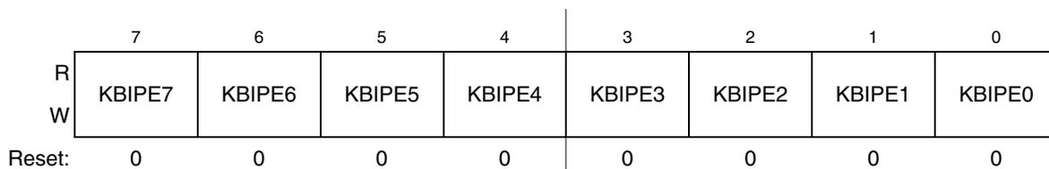
Figure 8-4. KBI Pin Enable Register
