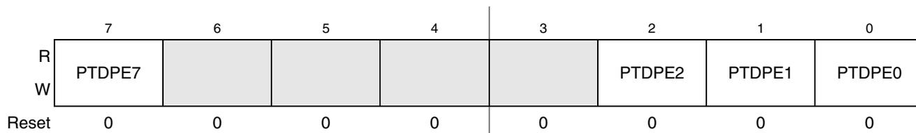
Figure 6-19. Internal Pullup Enable for Port D (PTDPE)
