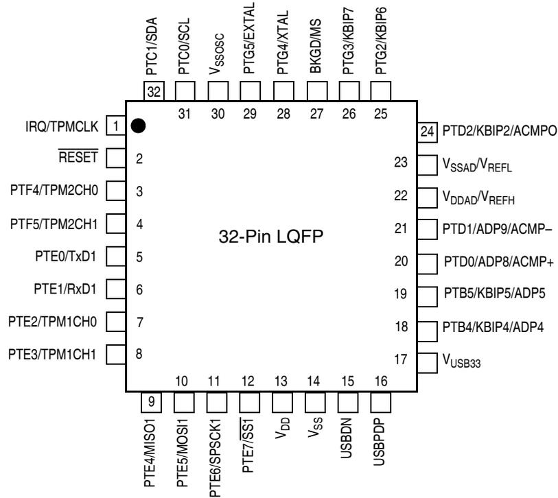
Figure 2-3. MC9S08JM16 Series in 32-Pin LQFP Package
