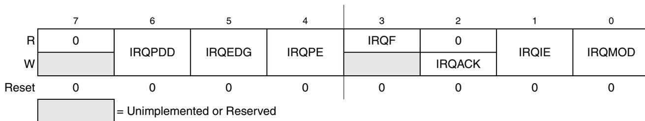
Figure 5-2. Interrupt Request Status and Control Register (IRQSC)
