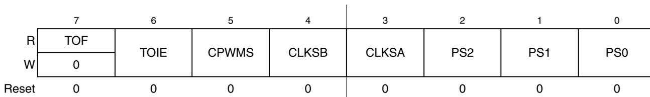
Figure 16-7. TPM Status and Control Register (TPMxSC)
