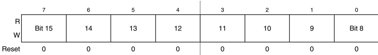
**Figure 16-10. TPM Counter Modulo Register High (TPMxMODH)**
