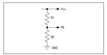
Figure 2. Setting the Output Voltage
