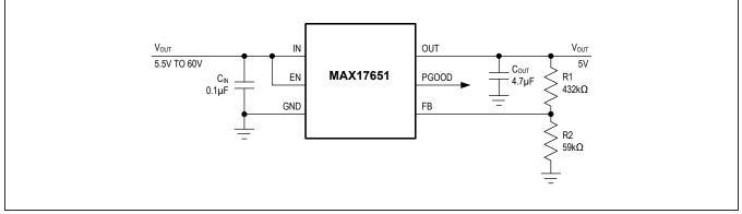
Figure 3. Application Circuit for 5V output
