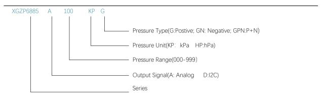
Note: 1. For specific output e.g 0.2~4.9V, signify output figure behind part number, e.g.: XGZP6885A250KPA0249
