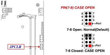
**Pin (7-8) Closed**: When Case open function pin short to GND, the Case open function was detected. When used, needs to enter BIOS and enable 'Case Open Detect' function. In this case if your case is removed, next time when you restart your computer, a message will be displayed on screen to inform you of this.
