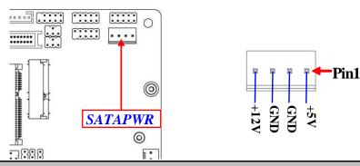
**Warning:** Make sure that Pin-1 of compatible SATA Power out connector is inserted into corresponding Pin-1 of **SATAPWR** connector to avoid possible damage to the board and hard disk driver!
