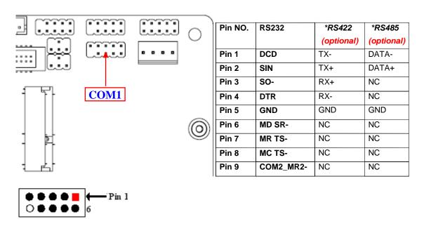
\*Note: COM1 header can function as RS232/422/485 port header. In normal settings COM1 functions as RS232 header. With compatible COM cable COM1 can function as RS422 or RS485 header. User also needs to go to BIOS to set 'Transmission Mode Select' for COM1 at first, before using specialized cable to connect different pins of this port.
