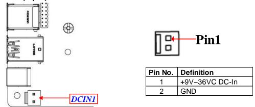
Warning: Find Pin-1 position before connecting power cable to this 2-pin power connector. WRONG INSTALLATION DIRECTION WILL DAMAGE THE BOARD!!
