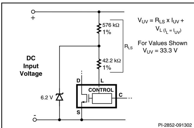
Figure 13. Line-Sensing for Undervoltage Only (Overvoltage Disabled).
