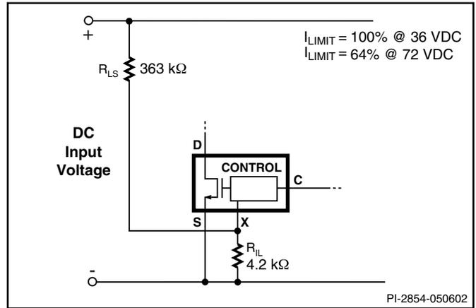
Figure 16. Current Limit Reduction with Line Voltage.
