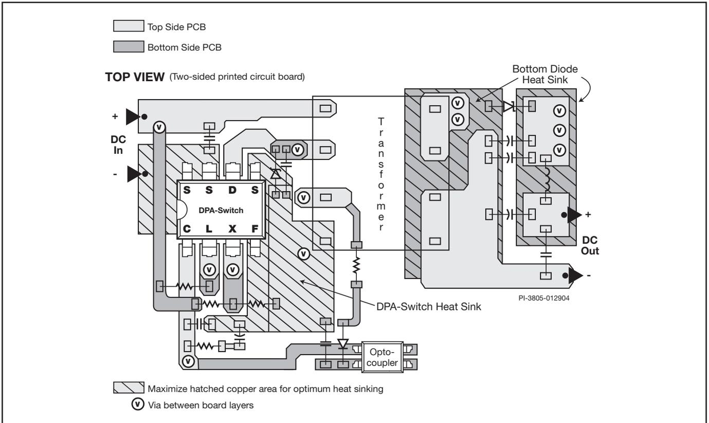
Figure 29. Layout Considerations for DPA-Switch using G Package.
