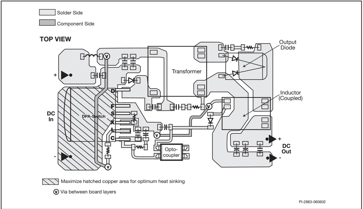
Figure 28. Layout Considerations for DPA-Switch using R Package.
