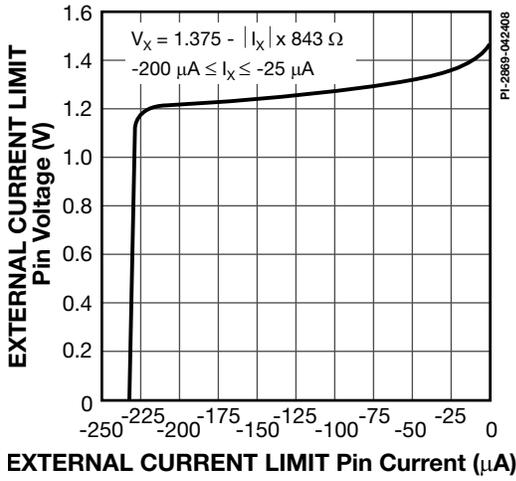
Figure 42. EXTERNAL CURRENT LIMIT Pin Voltage vs. Current
