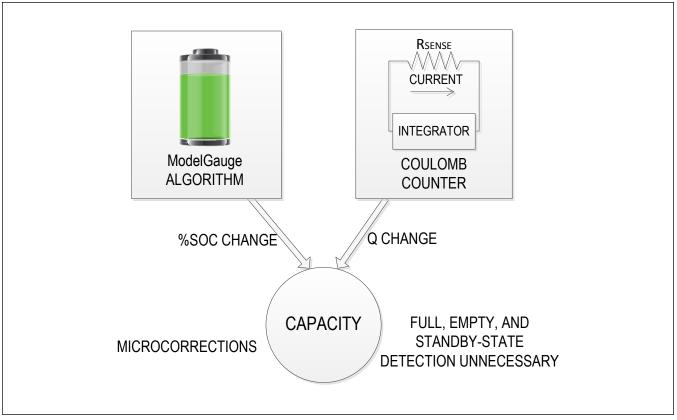
Figure 2. ModelGauge m5 Algorithm
