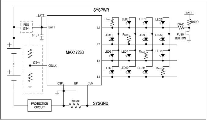
Figure 3. LED Charlieplexing Circuit
