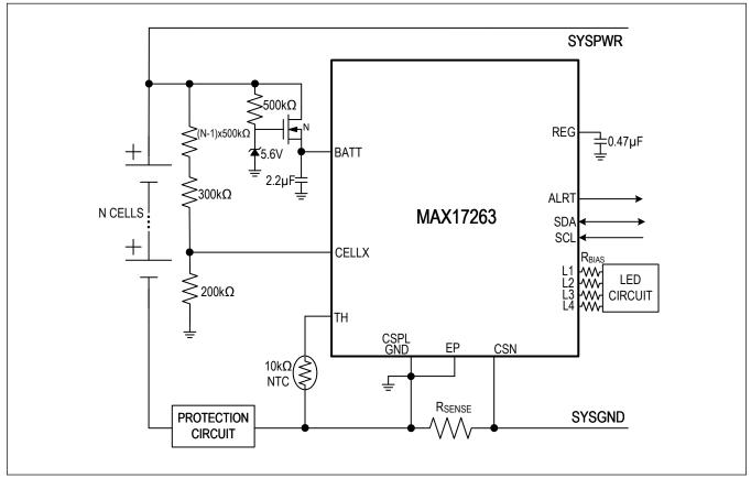
Figure 9. Multiple-Series Battery Typical Applications Circuit
